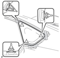
(3) Engage the 3 clips to install the quarter window glass (when a window without missing clips is used used).
