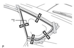
(1) Position the quarter window glass so that the matchmarks are aligned, and press it in gently along the rim (when a window with missing clips is used).
